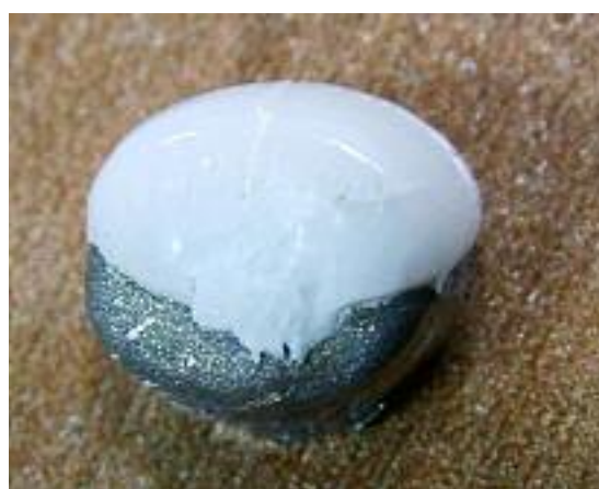
Figure 3. Mixed failure, loss of one second of the veneer material of lower first molar (Original magnification X10)
