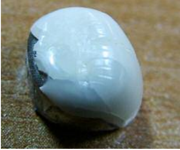
Figure 4. Mixed failure, loss of a third of the veneer material of lower first molar (Original magnification X10)
