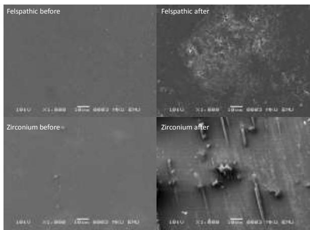
Fig 2: Surface roughness of the porcelains before and after air-flow polishing
