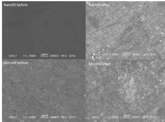
Fig 1: Surface roughness of the composites before and after air-flow polishing
