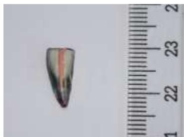
Figure 4. An example of dye leaked separated file.
